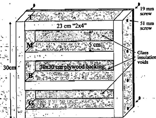
Fig. 1. Design of attic module. Nuptial chamber locations: T, top; M, middle; B, bottom; G, ground.
