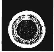
Figure 1. a) CT image showing water absorption after eleven days in end grain of spruce, starting on 12% MC. Light intensity corresponds to high amount of water. b) A crosscut of log from a dry site. The dark area is green heartwood and the light area sapwood. c). CT-image of a log from a wet site.
