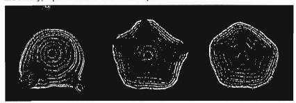
Pixel intensity will be a function of water content and other hydrogen bondings (lignin and cellulose) at every location inside the wood. Elements such as annual rings are clearly noticeable due to density changes between spring and summer seasons. Knots are also detectable since their water content and molecular structure are different from that of clear wood.
