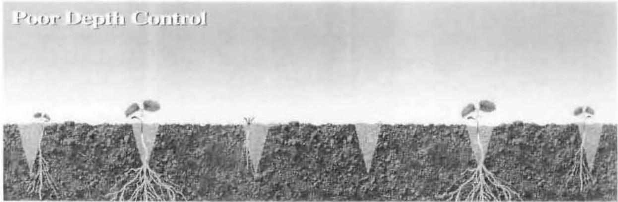
Poor depth control results in uneven emergence and wasted seed. Particularly in soybeans, the plant that emerges several days late, often produces less and sometimes nothing at all.
