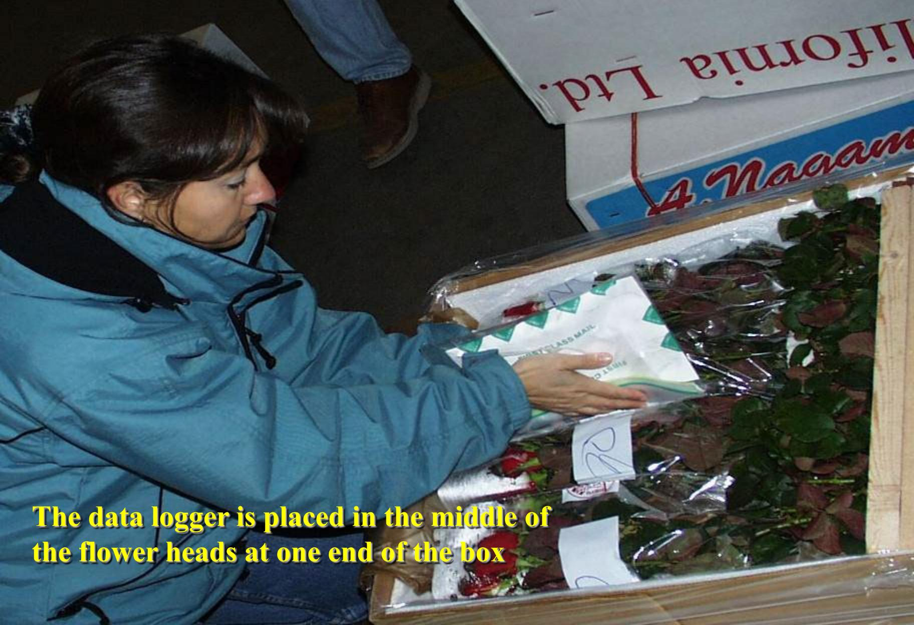
The data logger is placed in the middle of the flower heads at one end of the box
