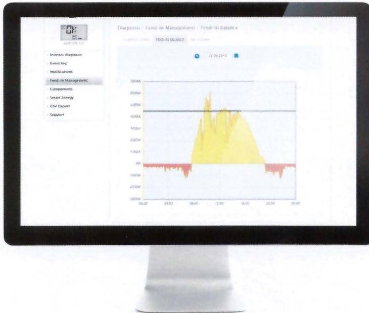
**Feed-in management - feed balance:** The times when there was a grid feed and when electricity was purchased from the grid can be seen at a glance in this graph. Negative values indicate that electricity was purchased from the grid and positive values that there was grid feed.
